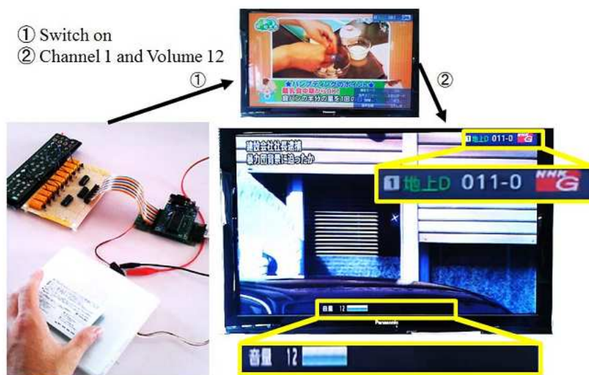
FIGURE 5. Demonstration of IC card operation
