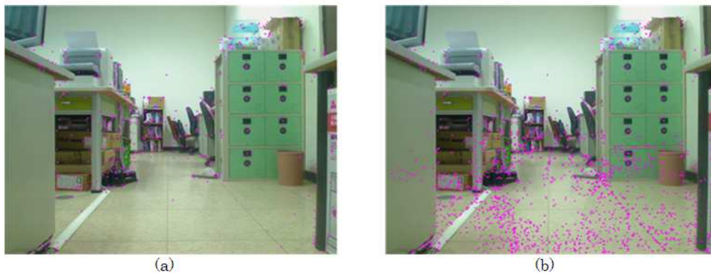
FIGURE 7. Feature scenes detected by (a) original SIFT and (b) proposed SIFT
