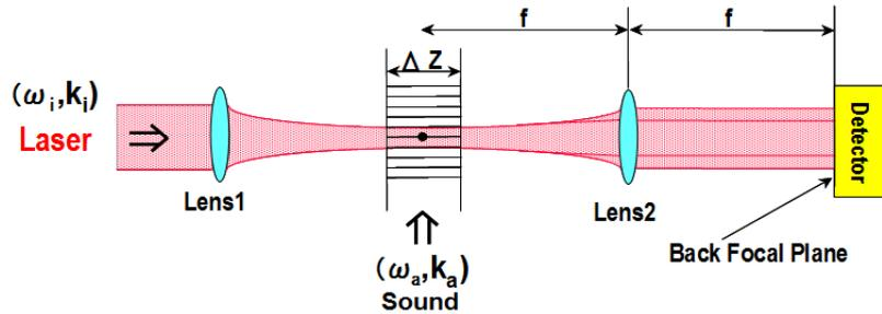
FIGURE 1. Optical setup for theoretical analysis
