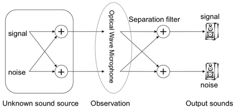
FIGURE 4. Blind source separation using an optical wave microphone
