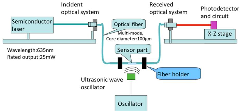
FIGURE 9. Optical wave microphone with optical fiber sensor
