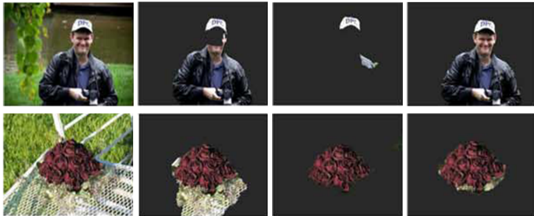
FIGURE 3. Results of object segmentation. The leftmost is the original image. The segmentation results from the second left to right are obtained from [4,5] and the proposed algorithm.
