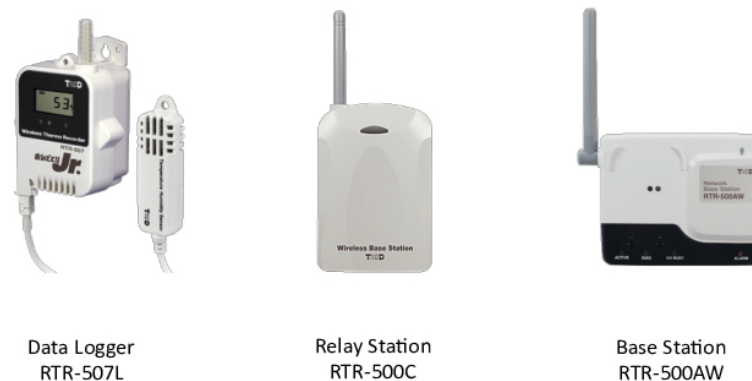
FIGURE 2. Wireless thermo-hygrometer equipments (T&D Corp.). Data logger (RTR-507L), relay station (RTR-500C) and base station (RTR-500AW). The data logger uses the platinum resistance thermometer sensor and electrostatic capacitance type sensor.
