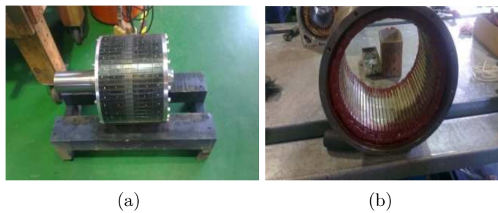
FIGURE 1. Photos of (a) the rotor, and (b) the stator for a PMSG
