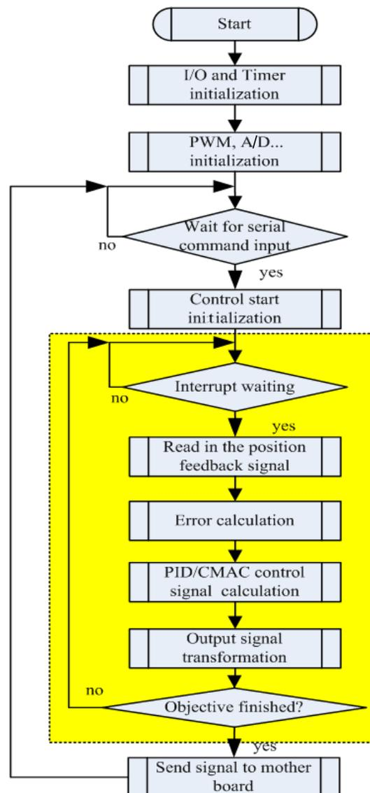
FIGURE 5. Main control program flowchart of proposed control driver
