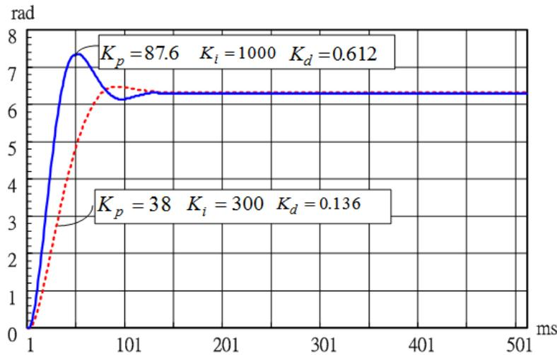
FIGURE 9. Time response for PID controller test
