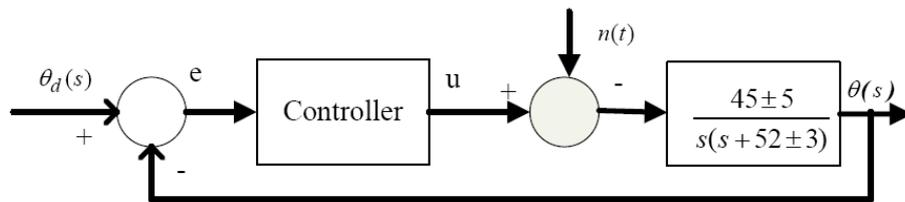
FIGURE 8. Control block diagram of DC servo control system
