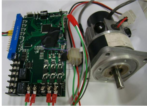
FIGURE 7. DC servo control system
