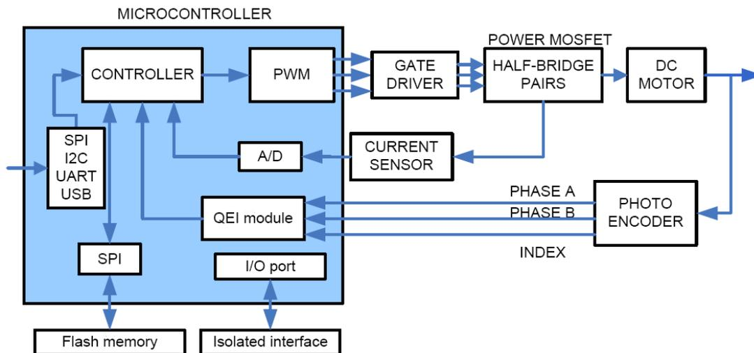
FIGURE 3. Block diagram of motion control driver
