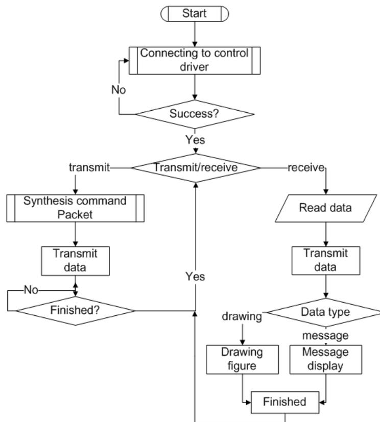
FIGURE 6. Communication program flowchart of PC terminal
