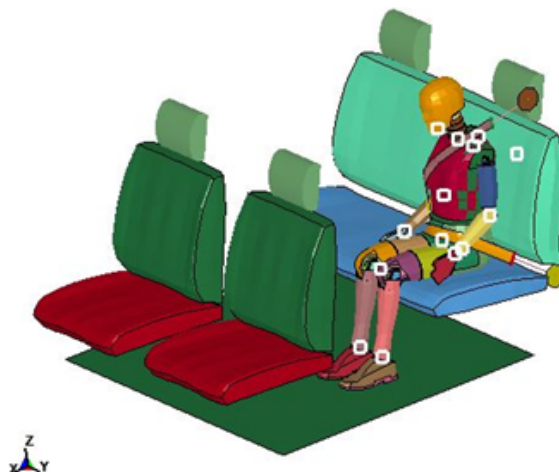
FIGURE 1. Finite element model of rear occupant restraint system
