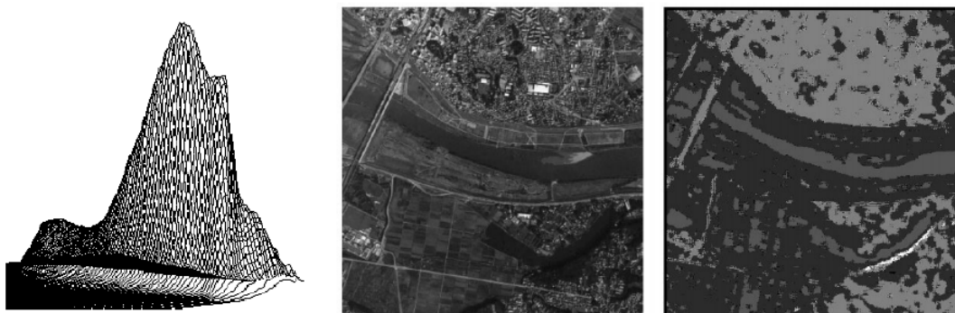
FIGURE 5. (Left) Histogram of (\alpha_{\min}, \alpha_{\max}) related to the aerial photograph of Toride; (Middle and Right) Original and segmented aerial photograph of Toride
